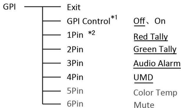
\*1 When "GPI control" is set to "On", the monitor can be operated through external GPI control unit.
